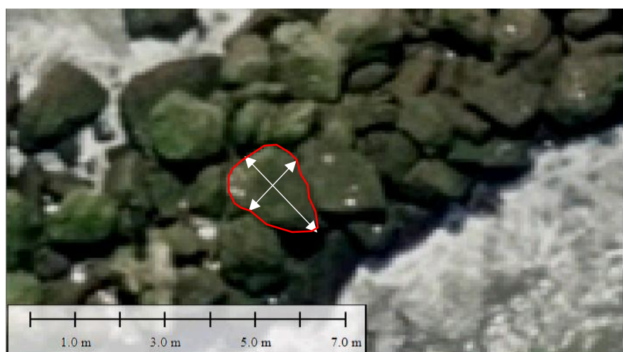
Figure 2.2: Method of measuring rock size
